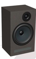
The SEAS A26 is a 2-way loudspeaker kit, using a 26 cm paper cone woofer and a 35 mm textile dome tweeter, in a compact 28 liter aperiodic enclosure. Carefully designed drivers with complementary response characteristics allow for a crossover network using only two components.
