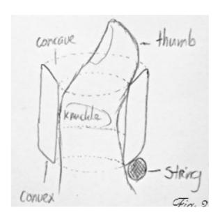
The ring must sit on the joint of the thumb and not be pushed past it. It feels counter intuitive and it seems the ring will easily slip. But when done right it is held firmly in place. Finding the right place requires some trial and error. Catch the bow string on the very end of the cylinder.
