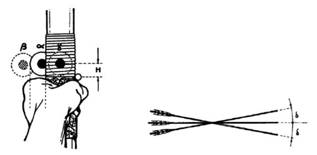
H depends on the draw weight of the bow and the weight of the arrow which together with the draw length and the distance from the target influence the inclination of the arrow d
